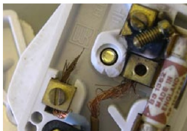
LIVE TERMINAL SCREW WELDED TO FUSE AND EARTH TERMINAL.
